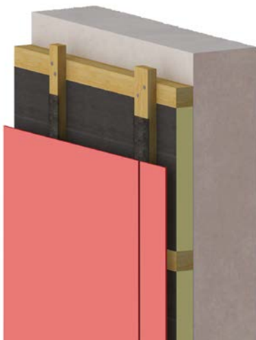
Structure with horizontal counter battens
